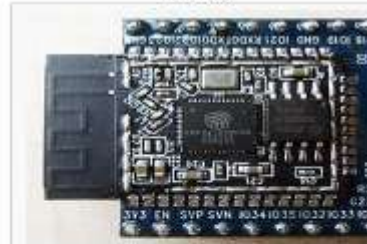
ESP-WROOM-32 module with ESP32-D0WQ6 chip
